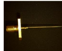
Figure 2: A custom micro-probe with a 0.25\ \mu\text{m} diameter Tungsten needle
